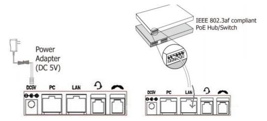
Note: If POE works, the phone doesn't need to connect to the AC power adapter. Make sure the Ethernet cable and switch/hub is POE compliant.
